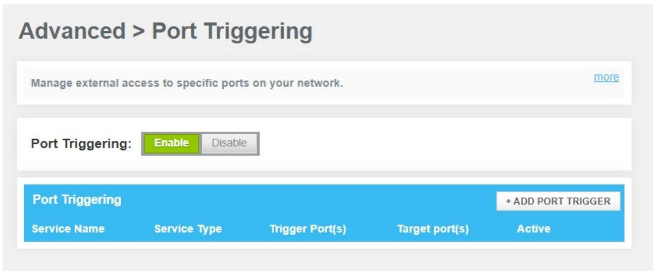
① **Port Triggering** Enable/Disable: Select Enable to manage external access to specific ports on your network.
